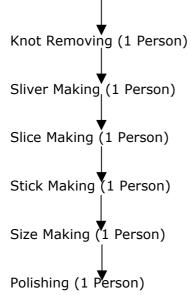
During stick making the stick making machine discharges heavy dust affecting workers and production. It was also noticed that most of the time workers involved in cross cutting & polishing were idle and they could be utilised on other machines reducing overall staff involvement. It was suggested that another stick making machine be installed leading to an increase of 50-60% or more in productivity with same number of workers.
